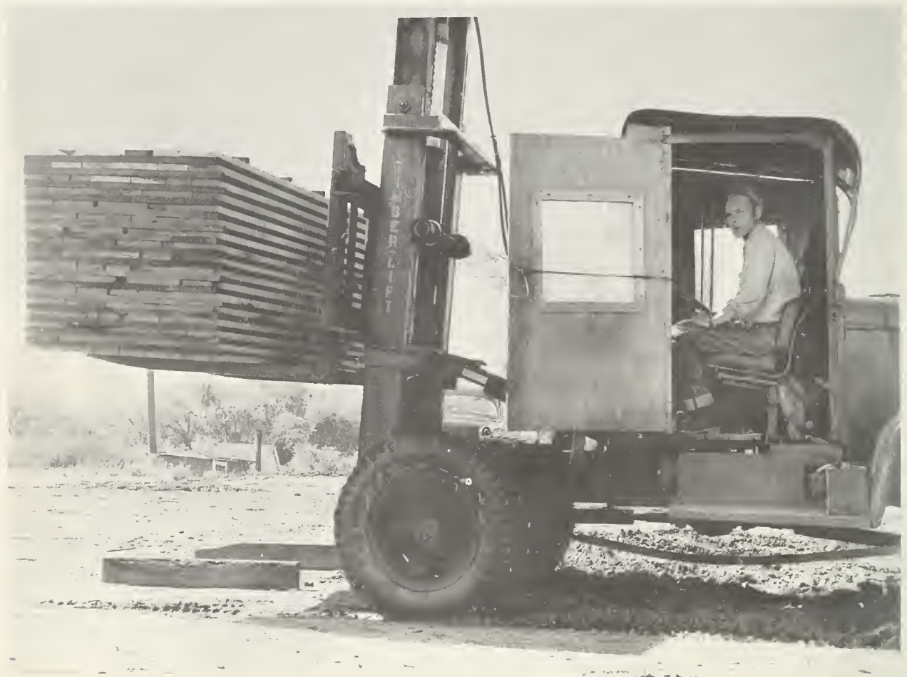
Figure 28. --Ordinary motor truck converted to fork lift.
